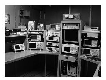
The ARRL Lab has a Faraday cage that allows it to perform measurements free of noise and interference. This photo shows the impressive array of test equipment the League uses to test equipment for *QST*'s "Product Review" feature.
