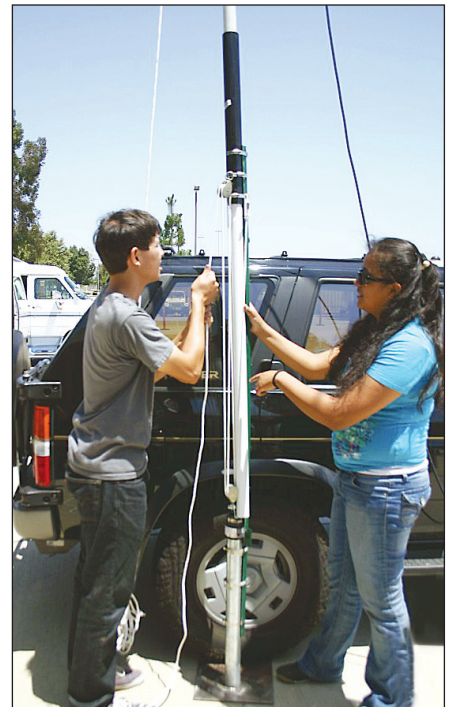
Chip Margelli, K7JA, designed a mast launcher for military masts like the one the Wilson AREC team uses. Margelli demonstrated it and we built one the next day. Here Philip Scholnick, KJ6MCD, and Carina Ochoa, KJ6MCB, are using the Margelli mast launcher for Field Day 2011.
