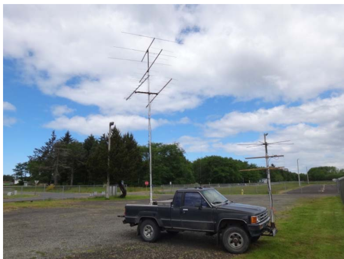
WW7D/R In Ocean Shores CN72 – The front stack is used while in motion while the rear stack is deployed at stops - note the homebrew antennas. (Photo provided by Darryl Holman, WW7D)
