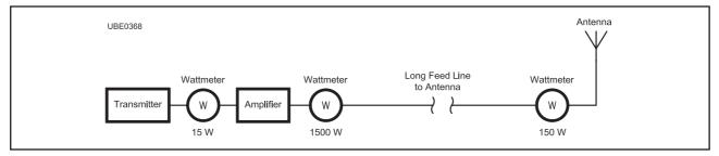
Figure E-1 — This diagram shows a power level measured at the output of an Amateur Radio transmitter. The diagram also shows power levels after the signal goes through a power amplifier and a long length of coaxial cable.
