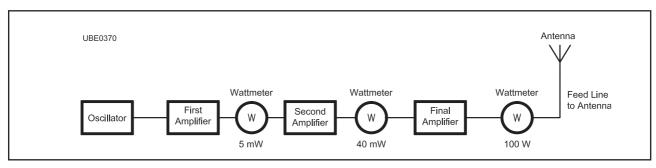
Figure E-3 — A simple amateur transmitter amplifies the signal from an oscillator and then feeds that signal to an antenna. It uses several amplifier stages. The input power to one of those stages is 5 milliwatts and the output from that stage is 40 milliwatts. The text describes how to calculate the gain of that amplifier stage.
