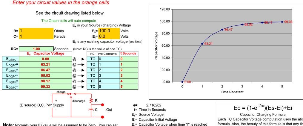
**Note:** Normally your **Ei** value will be assumed to be Zero. You can set Ei to be non-zero but it should be less than the Es voltage for the capacitor to be charging. You can do this, but think carefully about this new circuit dynamic. Also, be careful if you use negative voltage levels and the results that are presented.
