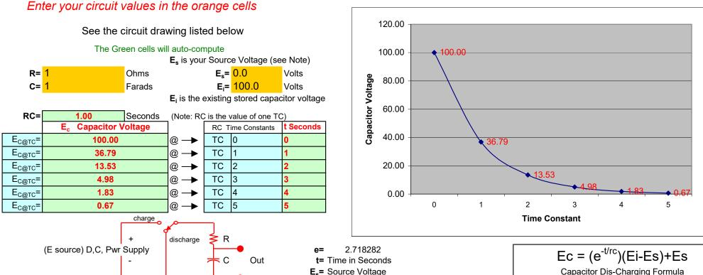
**Note:** Normally your **E**<sub>s</sub> value will be Zero. That is because there is no Power Supply in the above discharge circuit path as shown. You can make E<sub>s</sub> to be non-zero but it should be less than the E<sub>i</sub> voltage for the capacitor to be in discharge. If you do, your Non-Zero Es will be a new Es that you have virtually placed within the discharge circuit path. You can do this, but think carefully about the results and the new circuit dynamic you have now included.
