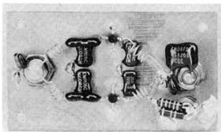
Fig 4—A 220-MHz version of the amplifier shown in Fig 3 can be built on unetched PC-board material.
