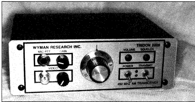
At left, the Wyman Research Tridon 2000, a 3-W transceiver. The latest addition to the line is the Tridon 2000H (right) capable of 12 W output. These units feature an attractive brushed-aluminum finish. (photos courtesy of Wyman Research)
